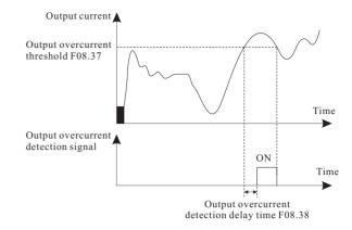
Figure 6-23 Output overcurrent detection
