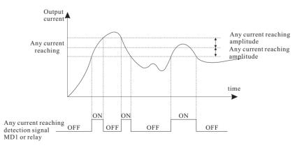
Figure 6-24 Any current reaching detection
