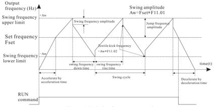
Figure 6-32 Swing frequency control
