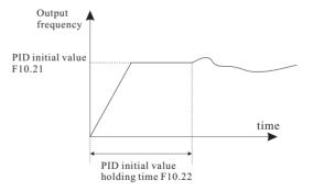
Figure 6-31 PID initial value function
