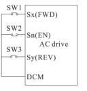
SW1 Sx(FWD) RUN SW2 Κ command Sn(EN) Forward AC drive OFF RUN Κ Reverse ON Sy(REV) RUN DCM
