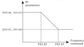
Figure 6-5 Relationship between running frequencies and PI parameters
