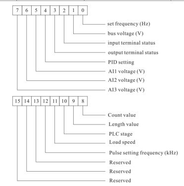
If a parameter needs to be displayed during the running, set the corresponding bit to 1, and set F07.05 to the hexadecimal equivalent of this binary number.
