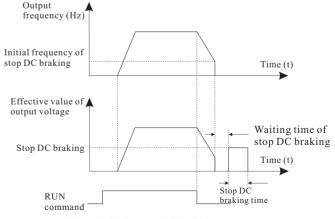
Figure 6-4 The stop DC braking process
