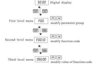
Figure 4-2 Operation flow chart of three-level menu
