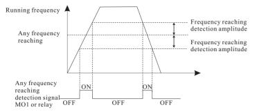
Figure 6-21 Any frequency reaching detection
