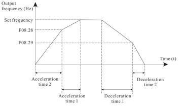
Figure 6-20 Acceleration/deceleration time switch over
