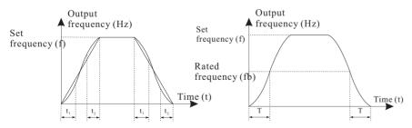
Figure 6-2 S-curve acceleration/deceleration A
