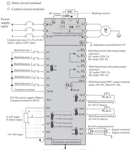
Extension card: I/O extension card, PG card (Relay extension card and V/I extension card can be customized as your request.)
