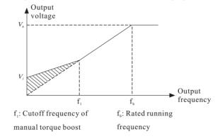
Figure 6-4 Manual torque boost
