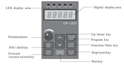
Figure 4-1 Schematic diagram of operation panel
