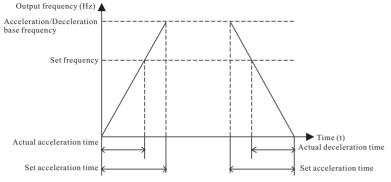
Figure 6-1 Acceleration/Deceleration time
