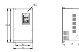
2.External dimension 2:wall-mounted/ floor combination housing
