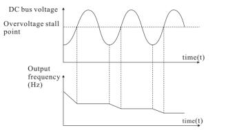
Figure 6-26 Diagram of the overvoltage stall protection function
