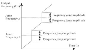
Figure 6-19 Diagram when the jump frequencies are valid during acceleration/deceleration
