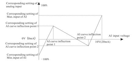
Figure 6-14 Curve 4 and curve 5
